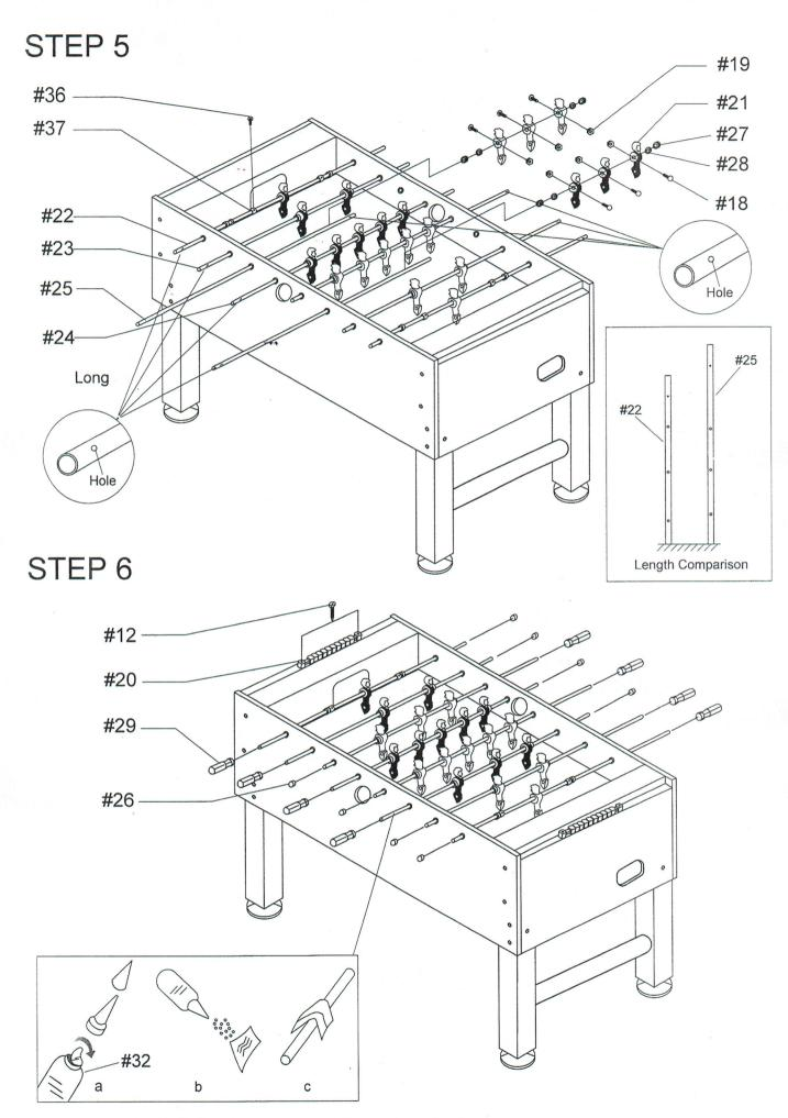
• Spray the lubricant(#32) into a clean, soft cloth and then use the cloth to wipe the player rods where they come into contact with the bearings. See above.
